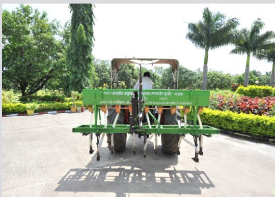
Fig- Soybean seed planter Features of the machine
