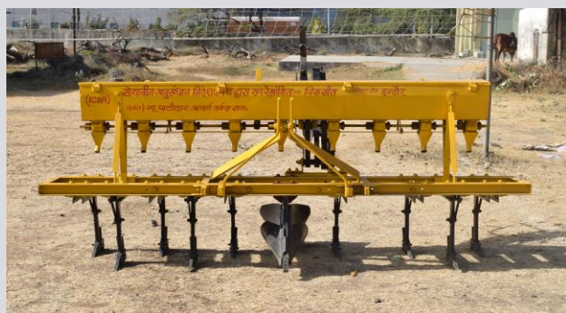
Fig 5 :Single bottom Broad Bed and Furrow (BBF) seed drill/planter.
